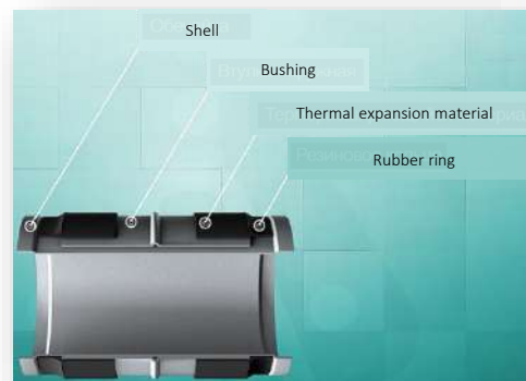
Bimetallic bushings for corrosion protection of welded joints of pipelines
