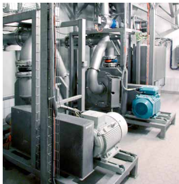
REKORD 630-2SSt grinding system for lactose
