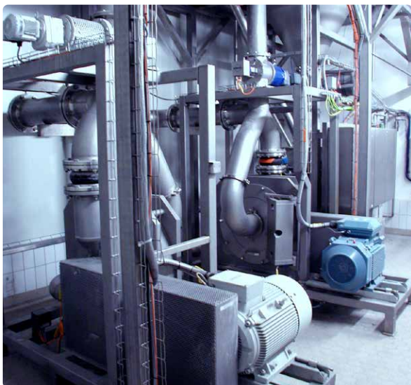
REKORD 630 GMP fine grinding system for lactose
