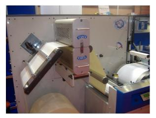
The adhesive rolls are changed by drawing out the top and/or bottom carriage as shown below
