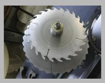
A common problem when cutting mineral and glass wool is the wear of the body under the carbide tooth. This consumable requires regular replacement. For this reason, maintenance costs are high, and the interruption of the production process occurs quite often. Constant friction on mineral wool affects the main saw blade very quickly. Such abrasion invariably leads to a loss of quality.
