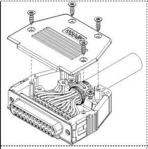
Place the hood lid on the hood assembly and secure it with the countersunk head screws, supplied.
