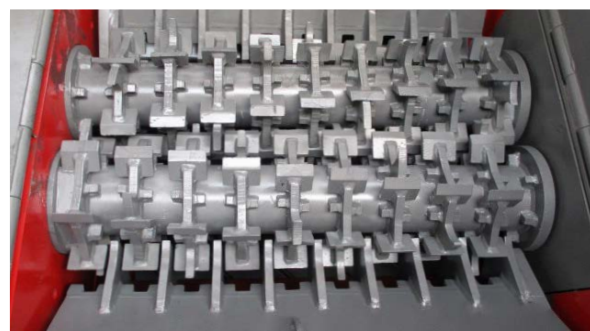
shredding shafts: 1,212 mm
