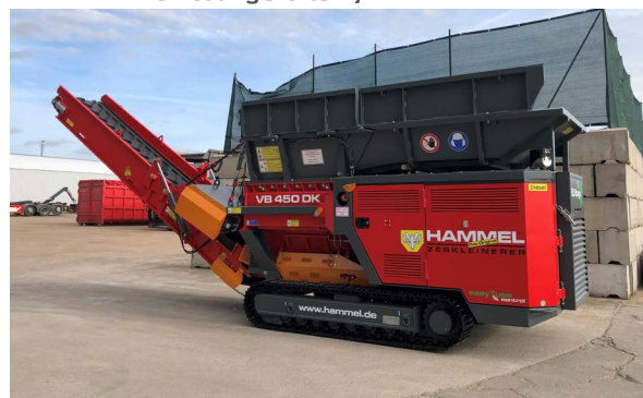
shredding shafts: 1,212 mm
